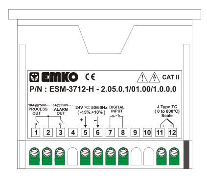
Device Label for J Type ( 0 ; 800 ) scaled, Thermocouple input, 24V ≂ Supply Voltage Input and SSR Driver Outputs
