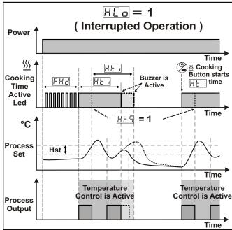
2-When cooking time parameter HE 1, if selection of temperature control and starting the cooking time parameter PHS = 1 (Temperature control starts at power on. Cooking time (Timer) can be started by pressing cooking ON/OFF button or when cooking time start/stop input is getting closed condition) is selected;
