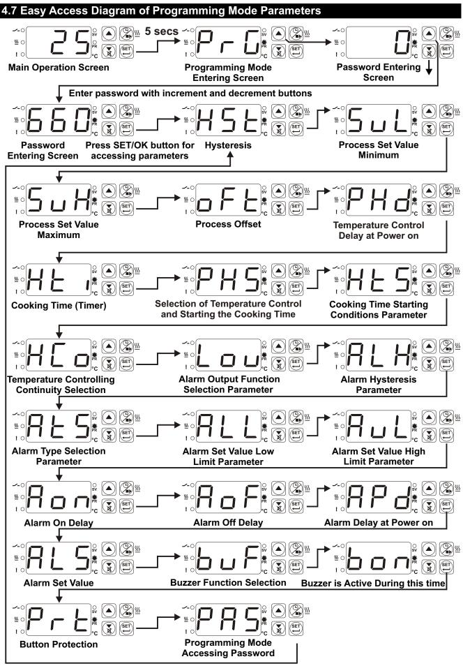
If no operation is performed in programming mode for 20 seconds, device turns to main operation screen automatically.
