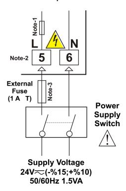
**Note-1 :** There is an internal 4R7 fusible flameproof resistor in  $24V \approx 50/60$ Hz supply voltage input.
