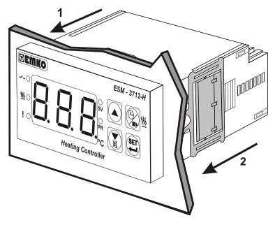
The unit is designed for panel mounting.
