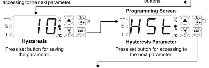
If no operation is performed in programming mode for 20 seconds, device turns to main operation screen automatically.
