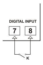
When K switch that is connected to the cooking time start/stop input, getting closed condition, cooking time (Timer) is started and cooking time active led becomes active. While cooking time (Timer) continues if K switch getting open condition, cooking time (Timer) is finished and cooking time active led lights off.
