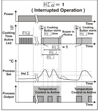
3-When cooking time parameter H = 1, if selection of temperature control and starting the cooking time parameter PHS = 2 (Temperature control and cooking time (Timer) can be started by pressing cooking ON/OFF button or when cooking time start/stop input is getting closed condition) is selected;
