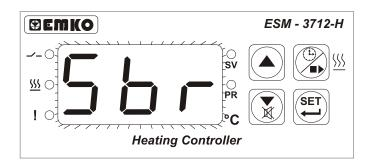
Probe failure in analogue input. Sensor connection is wrong or there is no sensor connection. When this message is on the screen, if alarm output function selection parameter Louis 2, alarm output becomes active and if buzzer function selection parameter buF is 3 or 4, internal buzzer starts to operate.
