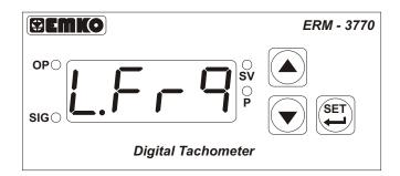
If the input frequency is lower than 0,07 Hz, then this screen will appear.
