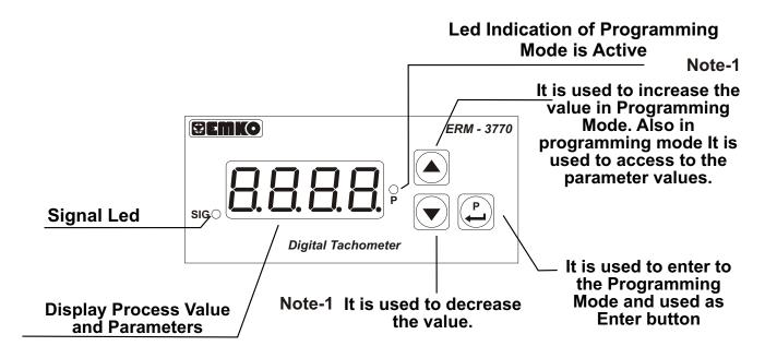
**Note-1:** If increment or decrement button is pressed for 5 seconds continuously, increment and decrement number become 10, if increment or decrement button is pressed for 10 seconds continuously, increment and decrement number become 100, if increment or decrement button is pressed for 15 seconds continuously, increment and decrement number become 1000.
