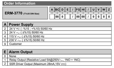
All order information of ERM-3770 Digital Tachometer are given on the table at left. User may form appropriate device configuration from information and codes that at the table and convert it to the ordering codes.
